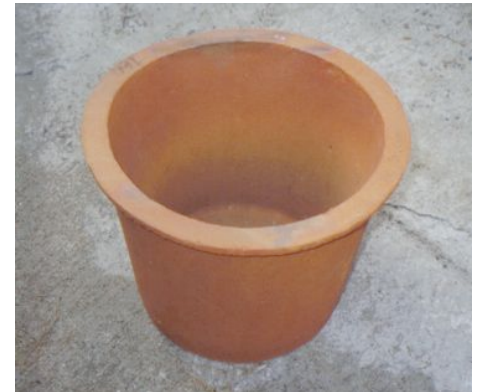
The Potters for Peace filter, locally produced in Nicaragua (CDC / D. Lantagne)
