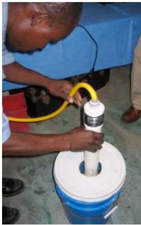
Manufacturing hypochlorite solution locally in a rural clinic in Haiti (CDC, D. Lantagne)
